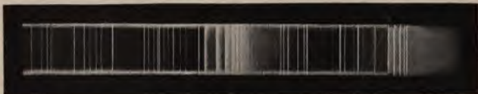
FIG. 48.—Violet and ultraviolet parts of spectrum of an arc lamp.
